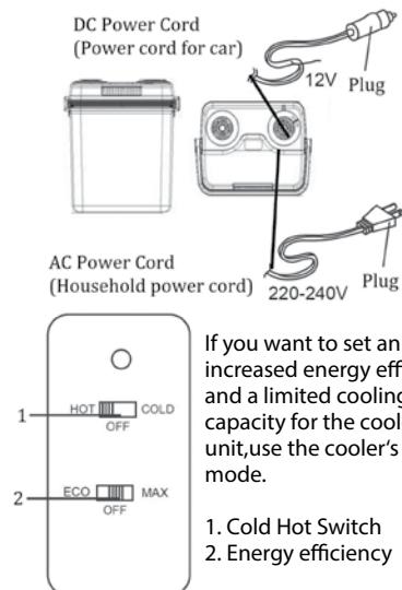
If you want to set an increased energy efficiency and a limited cooling capacity for the cooler unit, use the cooler's ECO mode.
